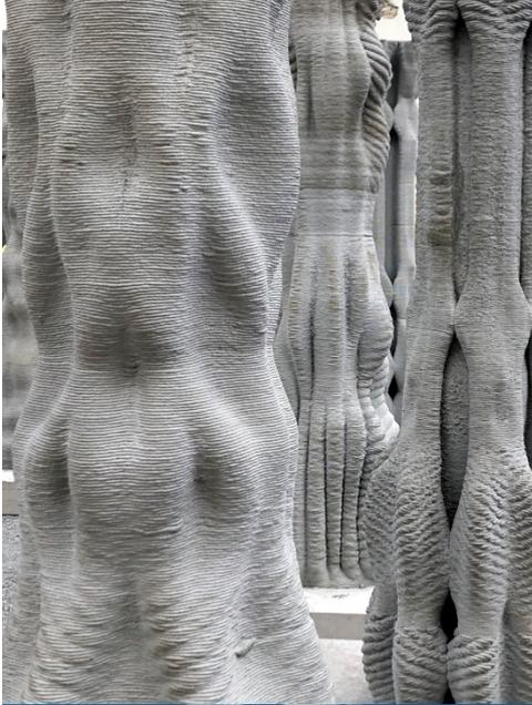
Details and surface texture of 3D printed concrete.
