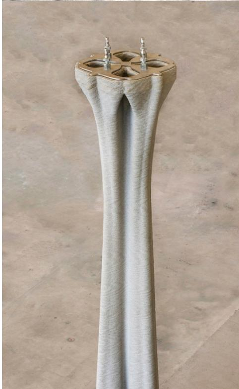
Post-tensioned system for a Concrete 3D Printed Colum, Scientifica 2019: Science Fiction Science Fact
